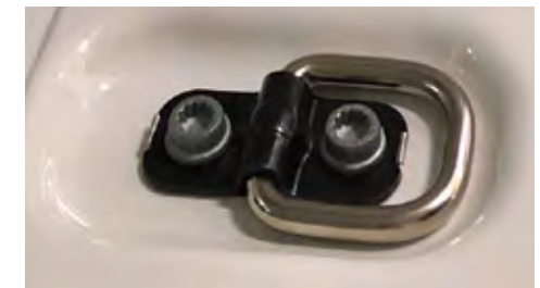
The lashing eyes are recessed to lie flush with the floor.
